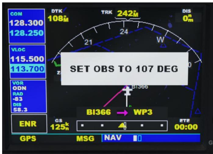
**Manually** set the HSI Course to the setting shown. The HSI will now give the correct indications in order to follow the flight plan leg.
