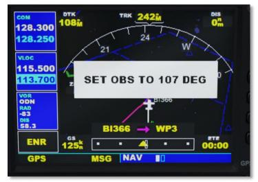
**Manually** set the HSI Course to the setting shown. The HSI will now give the correct indications in order to follow the flight plan leg.
