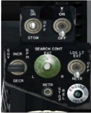
The internal lighting system consists of overhead dome lights that can be white or green and panel lighting in green. In flight only the panel lights are used. Note that the white dome lights are useful if you find the whole cockpit too dark, even during daylight hours. Do note that like many military cockpit the Huey panels are dark and offer little contrast.
