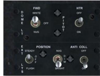
External lights include position (navigation) lights that can be set steady or blinking and bright or dim, the latter to be used with night vision equipment and anti-collision (strobe and beacon) lights. The landing light can be extended and retracted and accidental activation is prevented with a switch guard. The powerful search light can be retracted when not used and steered with the thumb switch
