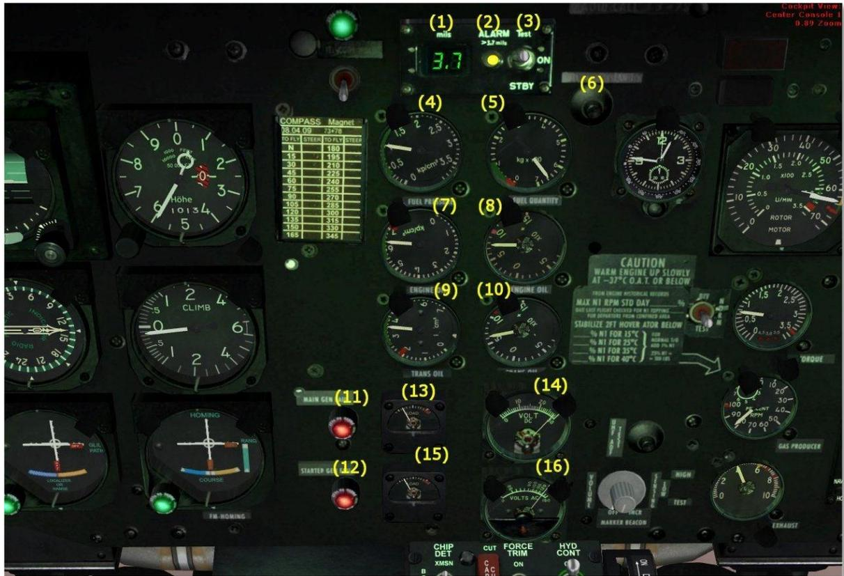
1. Engine vibration monitor readout
