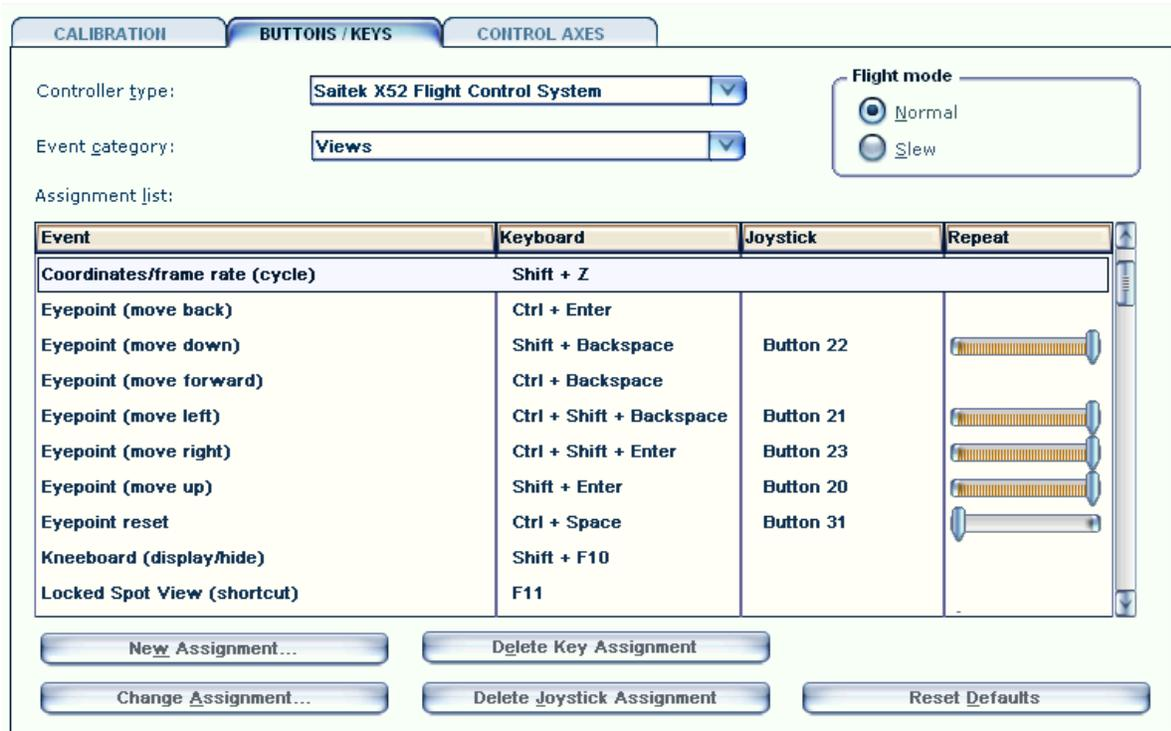
Shown above is the assignment of a secondary four-way switch on the joystick to the movement of the viewpoint. A fifth switch is assigned to a reset of the view because it is very easy to lose orientation. The movement is set to repeat, the reset is a single event.
