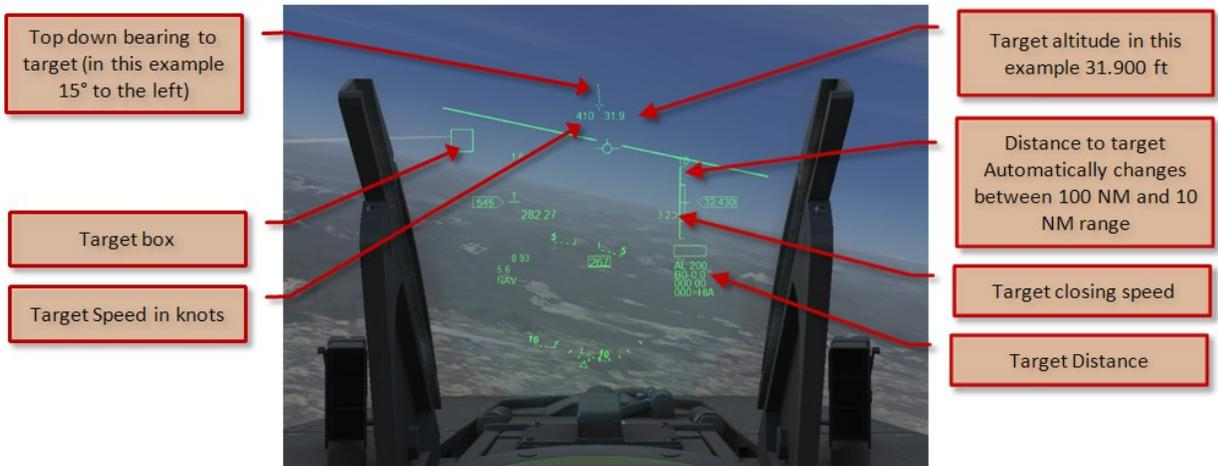
When the A-A button in the ICP is pressed a different intercept HUD is shown that makes it easier to close and track the locked target from shorter distances.
