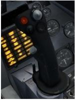
The side stick was one of the major innovations of the F-16. It was located to the side of the cockpit so the full arm of the pilot could be supported making high G maneuvers easier to control. Furthermore the stick was almost fully static. It did not move as other controls in aircraft did. It senses force applied to it and not movement. We added a tiny bit of animation to give the user some feedback though. There are no controls on the side stick for the FSX pilot.
