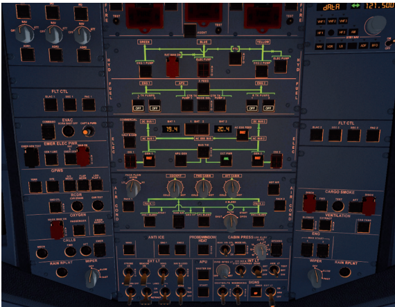
Overhead Panel before switching OFF both batteries
